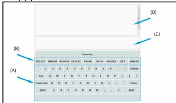
Figure 1. Main parts that make up the MyDB: standard keyboard (A), special keys (B), area to edit SQL commands (C), just above the keyboard, and an area for presenting the results at the top (D).
