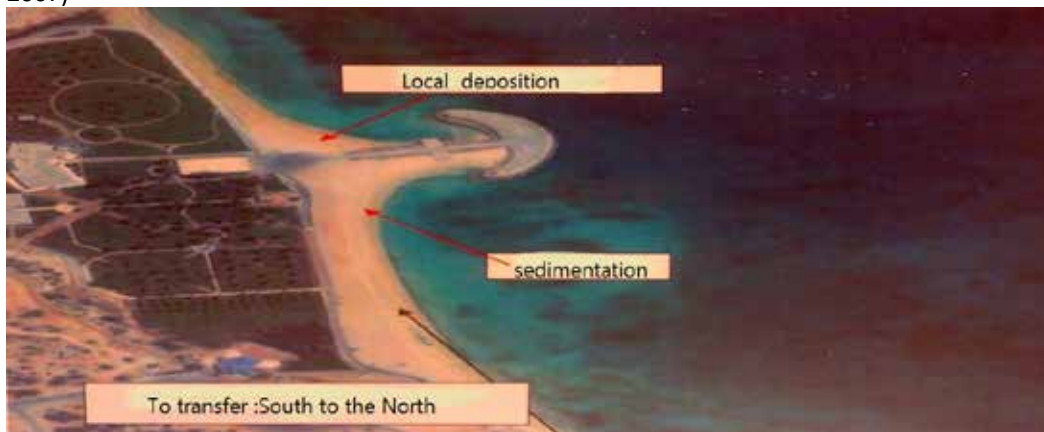
Figure 5 , Sedimentation around the Pavion Stone Pier (Source: Sazeh Pardaz Consulting Engineers, 2007)
