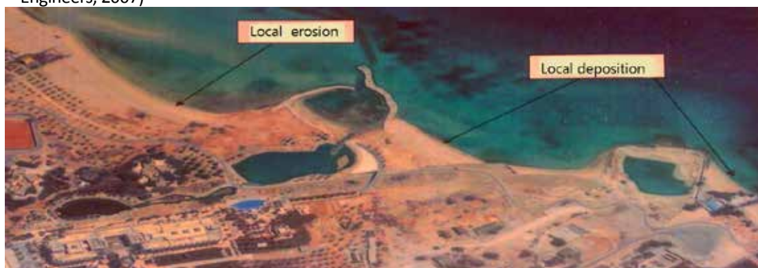
Figure 3 , Changes made on the coast opposite to Dariush Hotel (Source: Sazeh-Pardaz Consulting Engineers, 2007)
